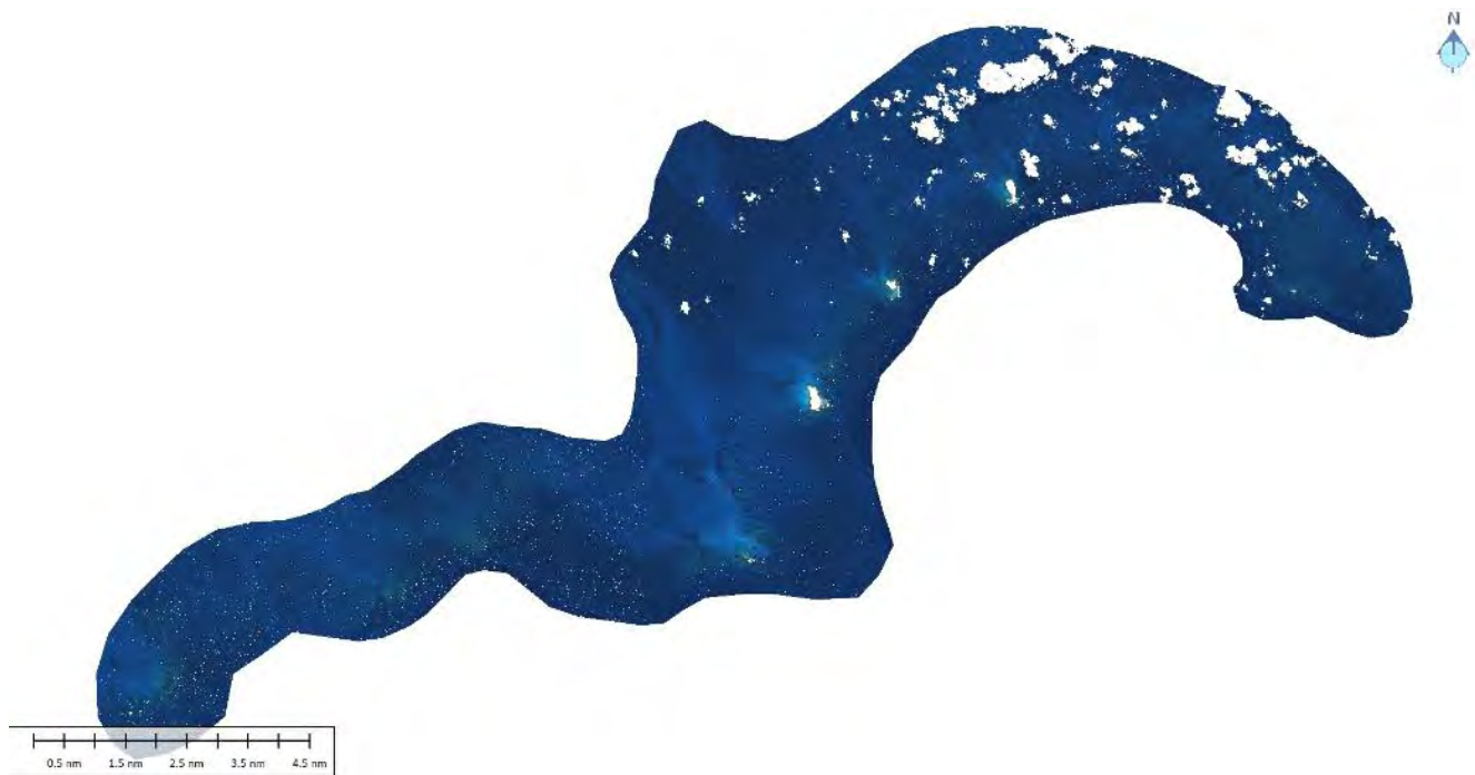
Figure 1 | True-colour (red, green, blue) WorldView-2 mosaic of Pedro Bank. The area encompasses approximately 300 sq. km. Water depths across the platform-top are in the range of 10-15 m and for this reason, the imagery appears blue in colour with only faint spectral differences representing changes in benthic character. Specialised spectral processing of the imagery was required to extract the seabed map. White areas in the imagery represent either clouds (north east of the mosaic) or a series of exposed sand cays that line the southern margin of Pedro Bank. Lacking a reef rim, the platform is subjected to open marine conditions and therefore represents an exposed hydrodynamic setting. North is top.
