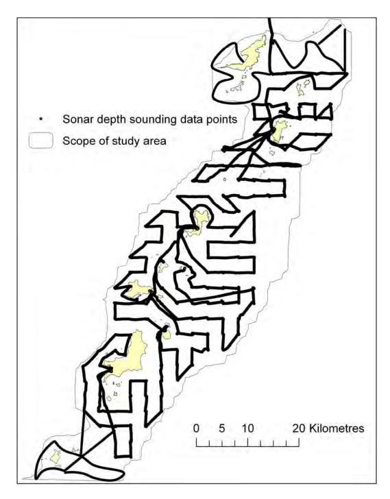
Figure 3-5 Survey cruise track showing continuous sonar depth sounding data collected to supplement existing bathymetric data for the Grenada Bank study area.
